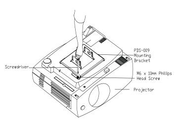
Using a screwdriver, secure the PDS-009 mounting bracket using four (4) M6 x 10mm Phillips Head screws. Do not over tighten these screws. Overtightening the screws may result in damaging the threaded inserts on the projector.
